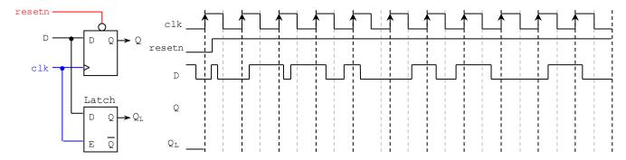
Complete the timing diagram of the circuit shown below. (5 pts)
