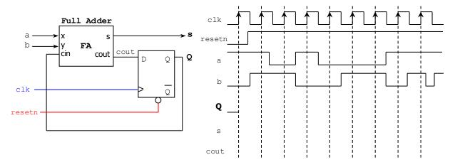
• Complete the timing diagram of the circuit shown below.  $Q = Q_3Q_2Q_1Q_0$  (9 pts)
